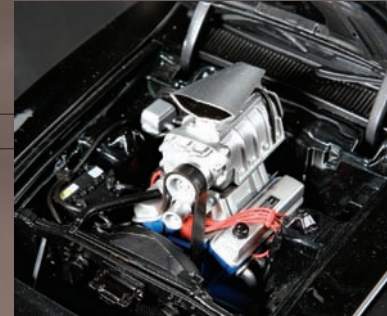
AUTOart made the model's engine more realistic than the original. This blower is actually hooked up—atop a tunnel ram for proper height.
